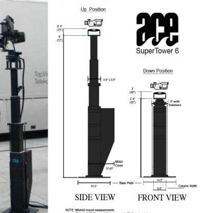
NOTE: Mitchell mount measurements Plate is 6.25" Square, Mitchell mount is 7" diameter circle Mount is 3" tall
